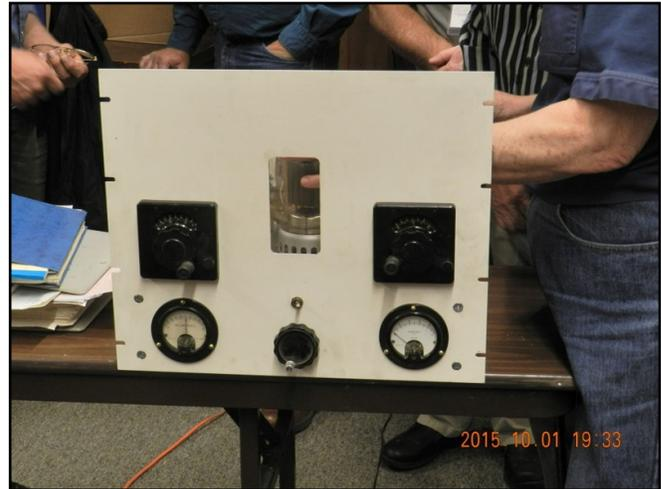
and a large inductor. Mike went through some designs for the Pi-networks used to impedance match the tube to 50 ohms. Mike plans on running about 4000 volts on
