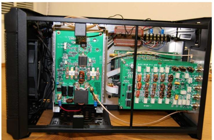
**Top view. 100w amplifier left, filters right.**
