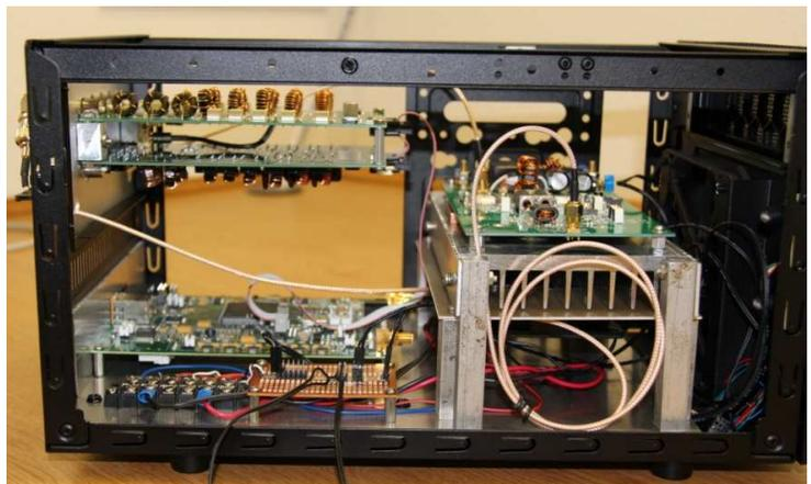
**Side view. SDR board bottom left, filters top left, 100w amplifier right.**
