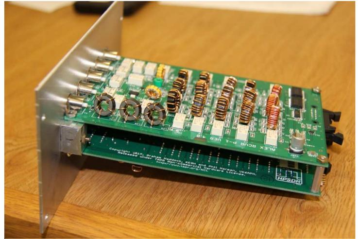
**Tx LPF and Rx HPF filters and antenna relays. Home machined mounting blocks.**
