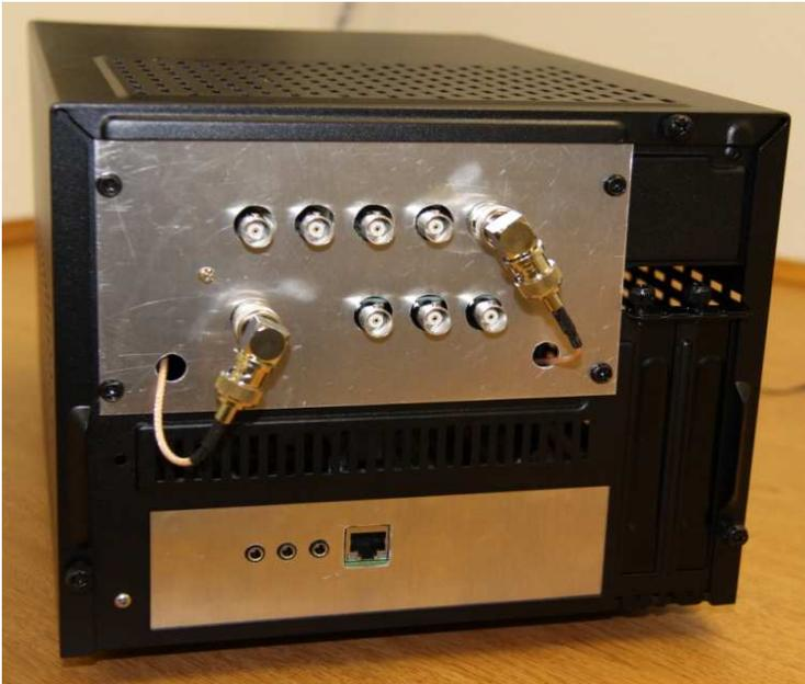
**Back of the radio showing multiple Antenna connectors, Microphone, CW Key, Speaker, and Ethernet Connectors.**
