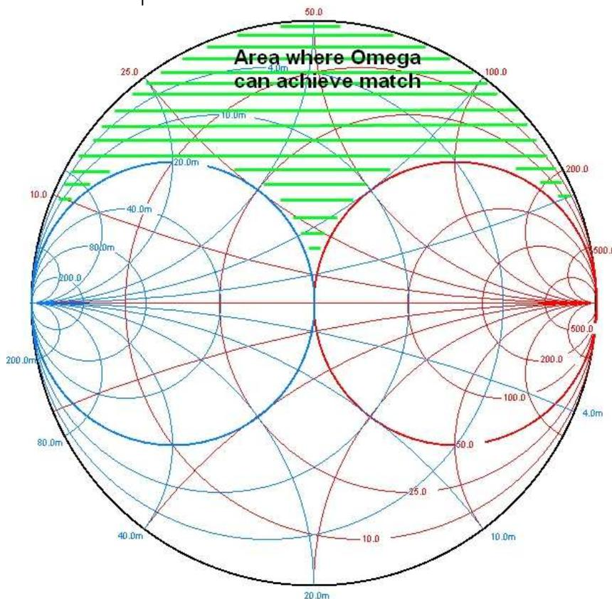
**The range of input impedances presented by the gamma rod that can be matched to 50 ohms with an omega match is the green shaded area in the upper portion of the chart.**
