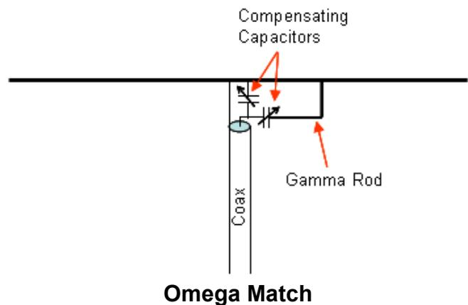
wavelength and thus it could prove difficult to find a 50-ohm tap point that allows the gamma match to achieve a 50-ohm match. In this case, an additional variable capacitor can be added to substantially increase the range over which the match can be
