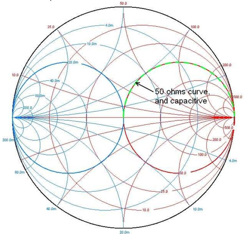
**The range of input impedances that can be matched to 50 ohms with a gamma match is the half-arc shown by the dashed green line.**
