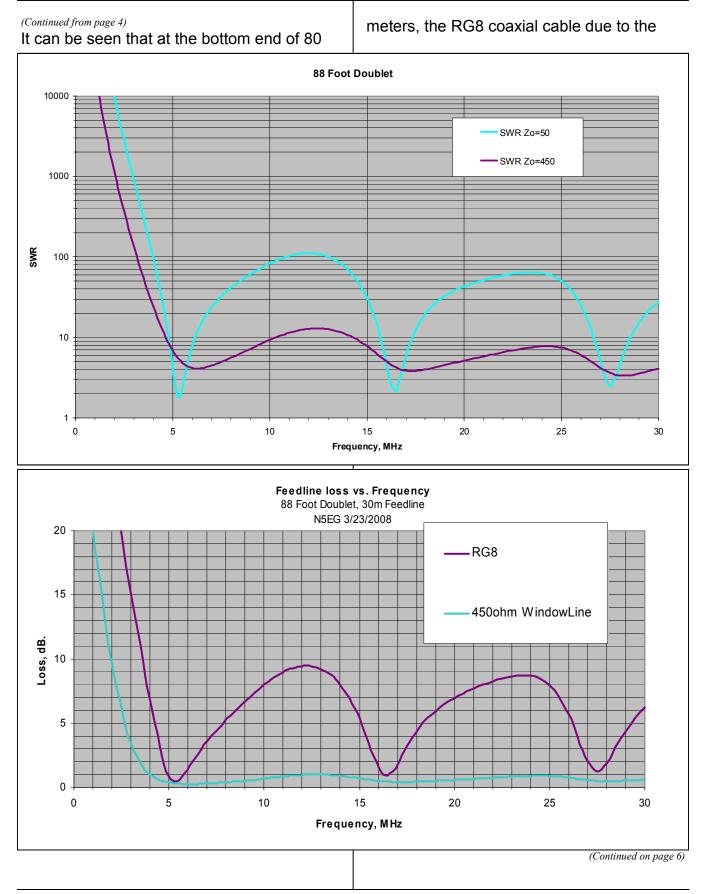
very high SWR has about 12 dB of loss, while the 450 ohm ladderline has about 2 dB of loss. While neither is terrific, the ladderline is far superior in this application. The coaxial cable would be a good choice if operating this antenna at one of it's near-resonant points. Unfortunately none of those are near any amateur bands.
