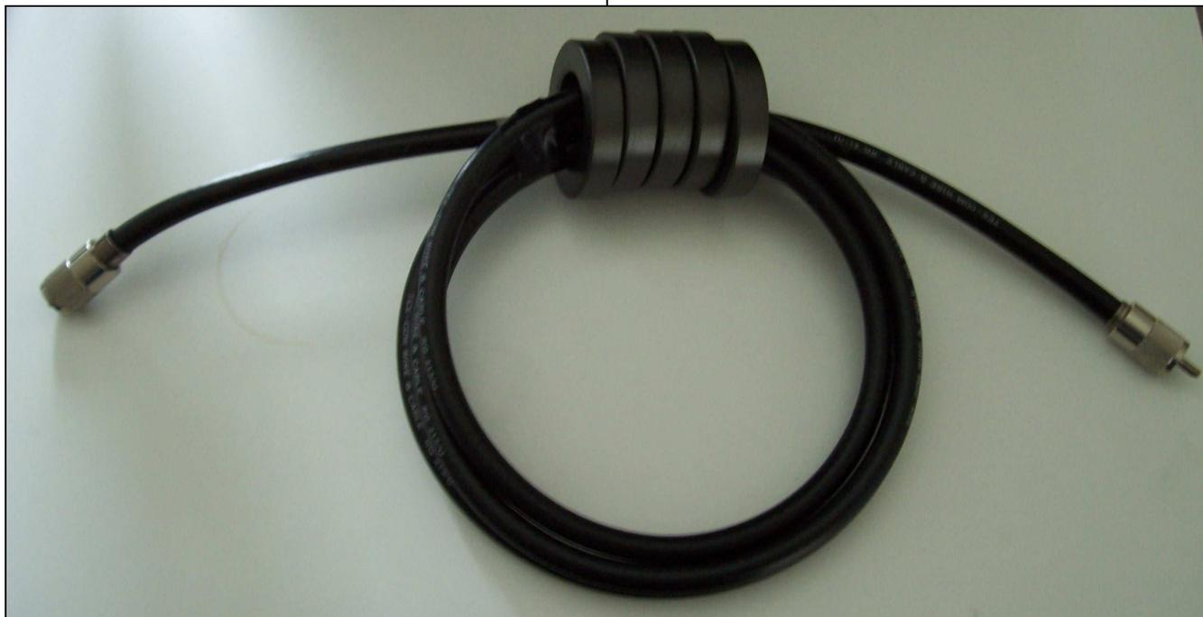
**Figure 1—1:1 Current Mode balun constructed from RG-213/U**
