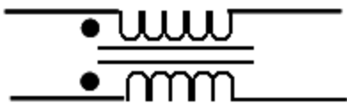
Figure 3—1:1 Current-mode balun. Each winding has the same number of turns, and the turns are bifilar or coaxial.
